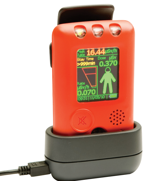
Portable dock: for charging and transferring data.
