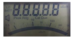
For the following two seconds, the next "CAL DUE" date will show using a MM/YY format.
